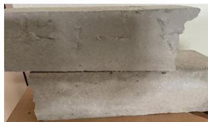
Figure 4. Failed Beam Specimen from UTM
