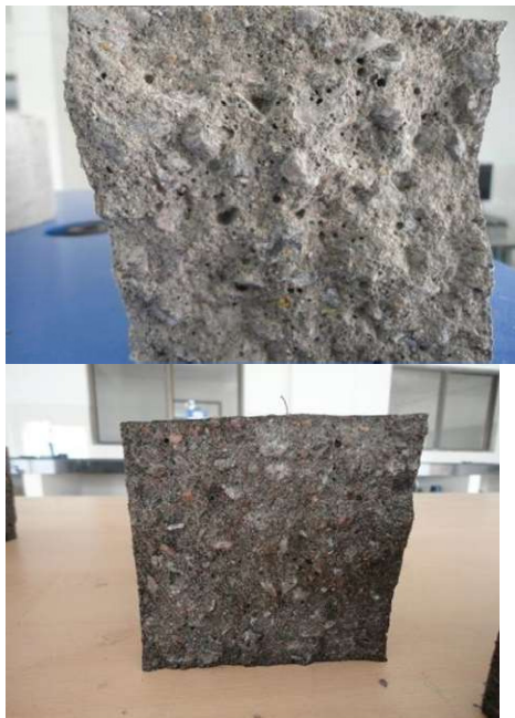
Fig. 4.10: Cross section of beam specimens of SCC mix with NS and CS
