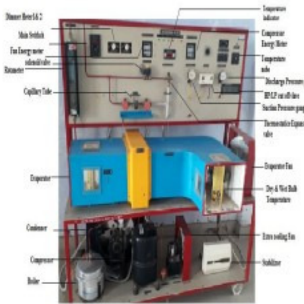
Figure.2 Physical experimental test rig of air conditioning
