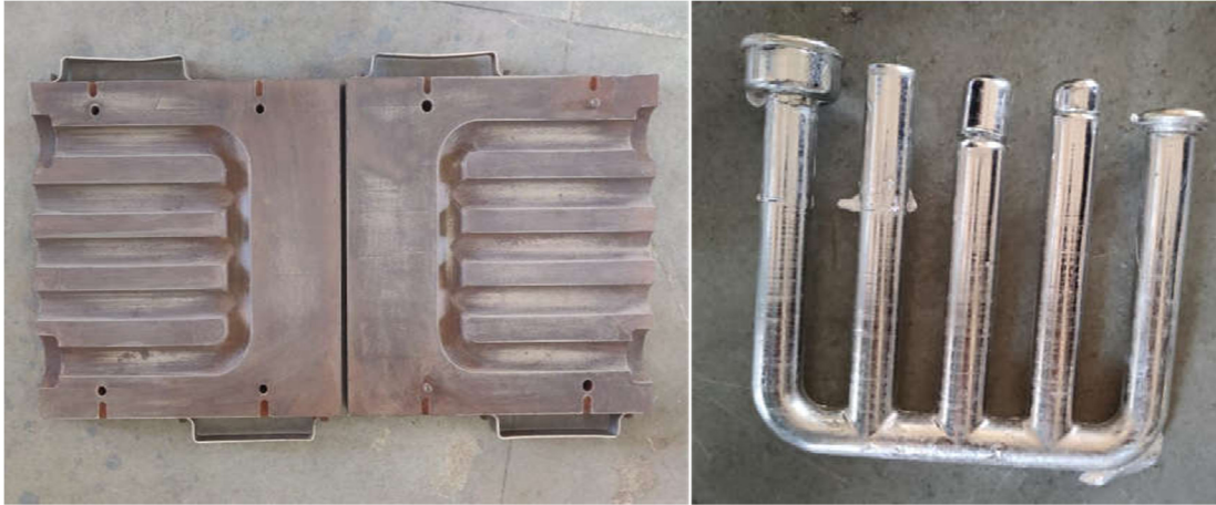
Fig.2 (a) Metallic Die (b) Casting after solidification
