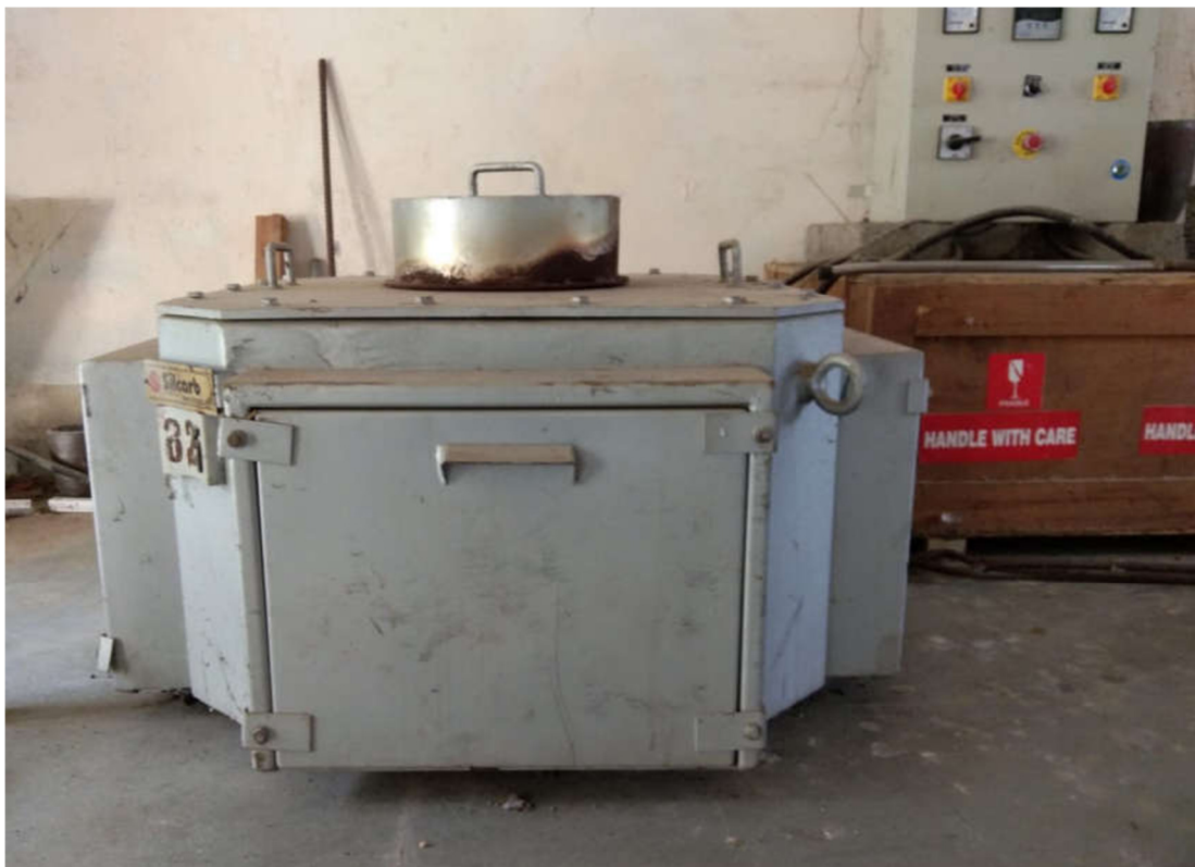
Fig.1 Electric resistance furnace with controll unit.
