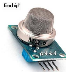
Fig. 4 Carbon Monoxide (CO) sensor MQ 6
